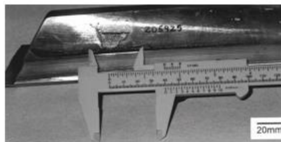
Fig.2: Representative case of a badly damaged pinion tooth surface.
