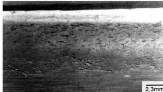
Fig.3: Detailed view of the contact line and neighboring regions of counterpart bigger gear viewed with a binocular stereoscope (microscopic pitting).
