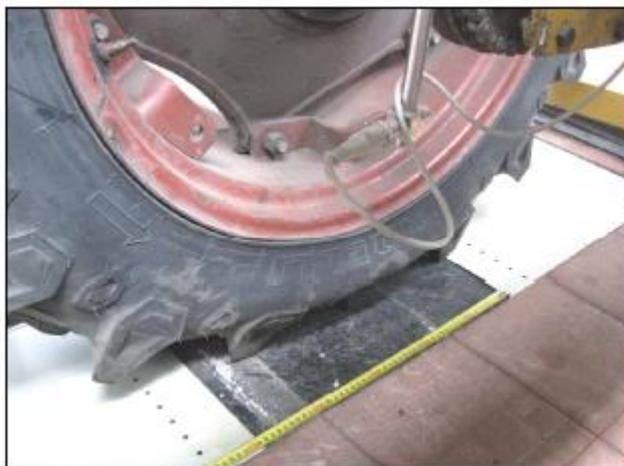
Fig.1: *Measuring tyre contact length*
