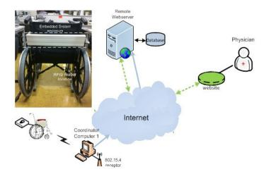
The smart sensing part is accomplished by a network of smart sensors (IEEE 1451.4)[6] that are embedded in a wheelchair, thus creating the concept of a smart wheelchair. The smart sensors are connected to an embedded platform based on microcontroller (MCU) that performs the signal
