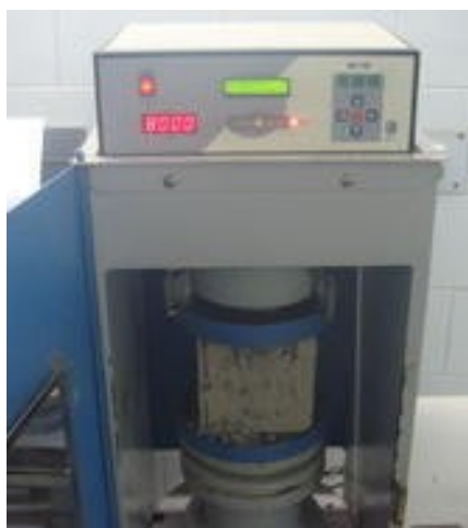
Fig: testing of cubes and cylinders
