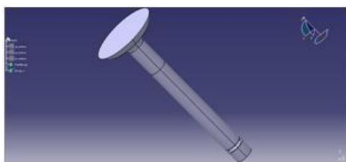
Fig 3.2 CATIA model of bi metallic valve
