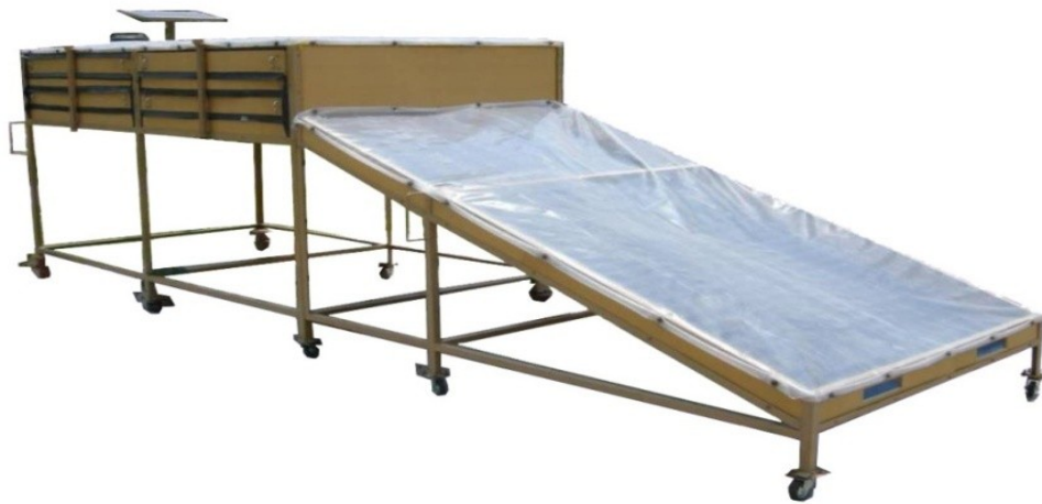
Figure 2.2 Fabricated solar dryer
