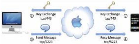
Figure 1: High-level operation of iMessage.
