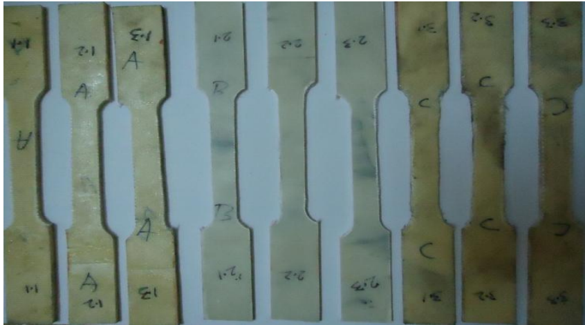
Fig.02 Tensile Strength testing specimens
