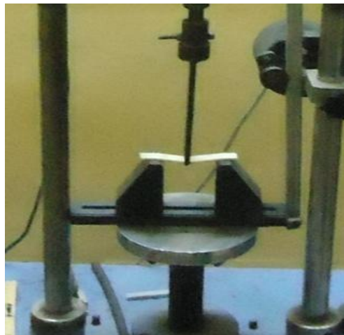
Fig. 03 Flexural testing setup
