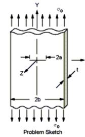
Fig. 1. Model of plate with center crack
