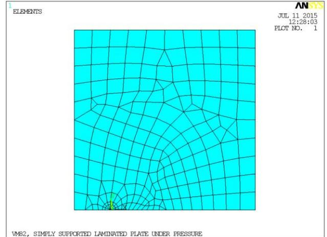
Fig. 7. FE Model of plate with center crack of a/b=0.2
