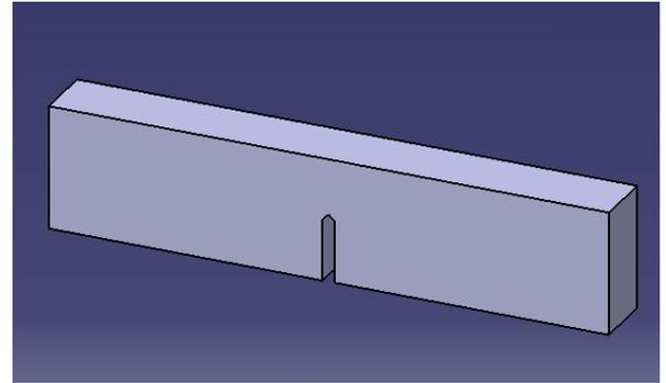
Fig. 13. Model of plate with 3-point bend
