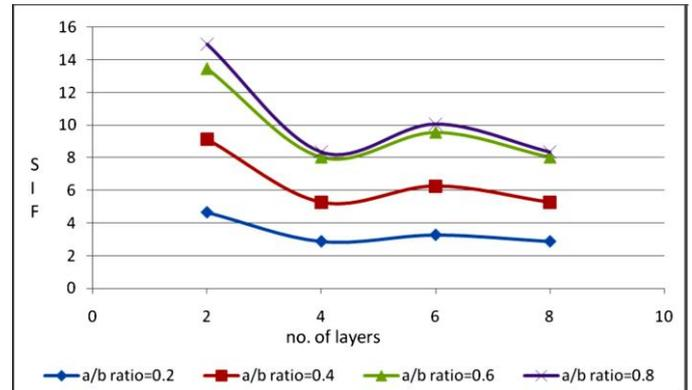
Fig. 19. Variation of Stress Intensity Factor (SIF) with increasing number of layers
