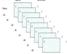
Fig. 6. Material with 8 layers
