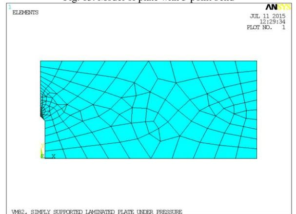
Fig. 14. FE Model of plate with 3-point bend
