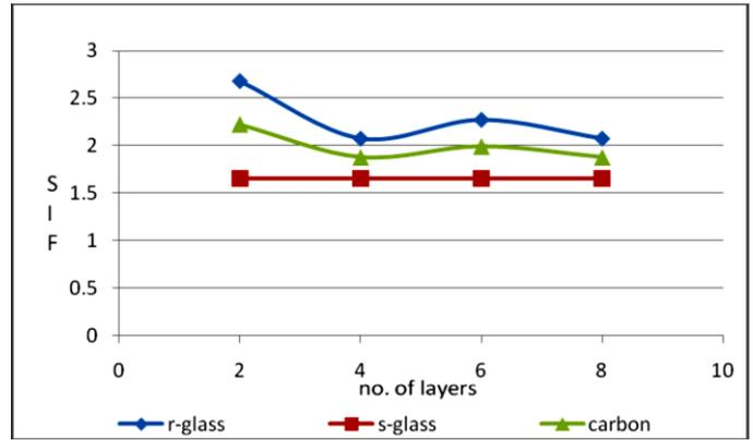
Fig. 30. Variation of Stress Intensity Factor (SIF) with increasing number of layers
