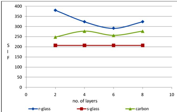
Fig. 25. Variation of Stress Intensity Factor (SIF) with increasing number of layers
