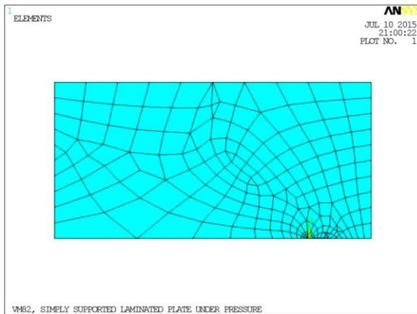
Fig. 11. FE Model of plate with edge crack of a/b=0.8
