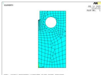
Fig. 12.(b) CT Developed Model
