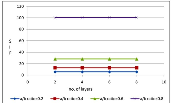
Fig. 23. Variation of Stress Intensity Factor (SIF) with increasing number of layers
