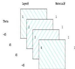
Fig.4. Material with 4 layers
