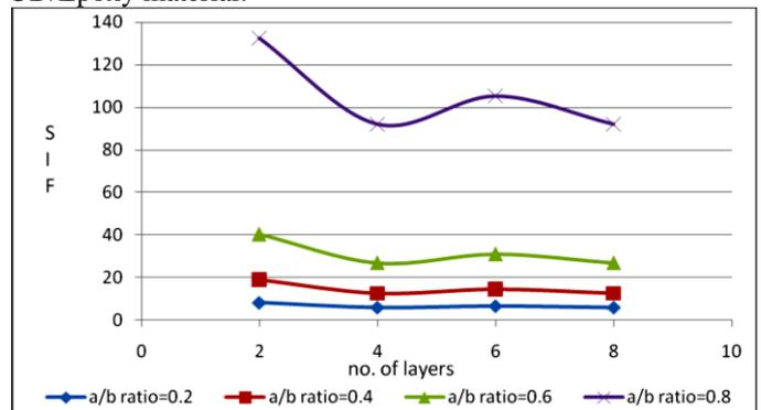
Fig. 24. Variation of Stress Intensity Factor (SIF) with increasing number of layers.
