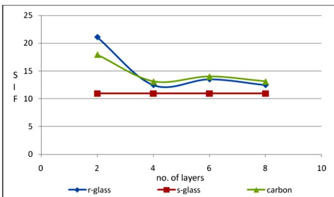
Fig. 26. Variation of Stress Intensity Factor (SIF) with increasing number of layers
