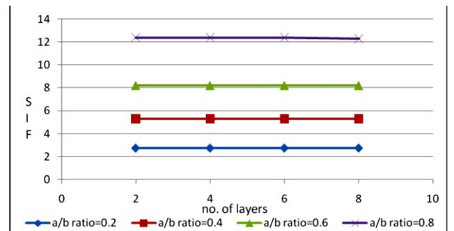
Fig. 20. Variation of Stress Intensity Factor (SIF) with increasing number of layers
