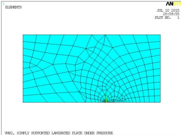
Fig. 10. FE Model of plate with edge crack of a/b=0.6
