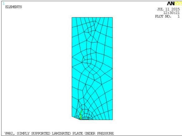
Fig. 16. FE Model of plate with V-notch
