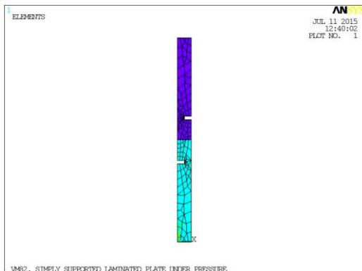
Fig. 18. FE Model of plate with double notch
