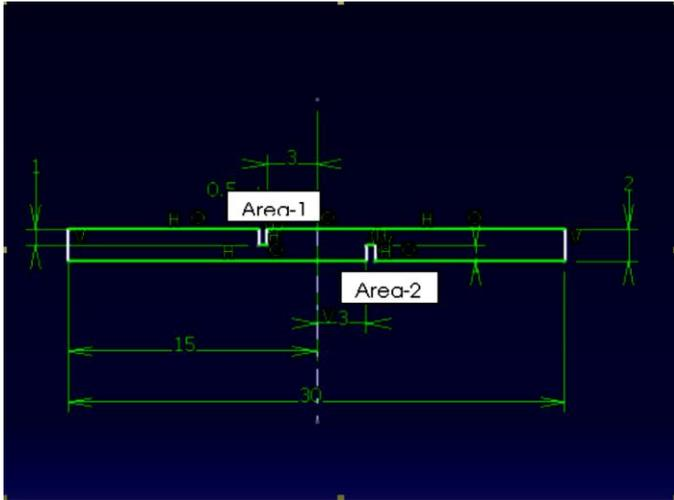
Fig. 28. Model of plate with double notch showing the two areas
