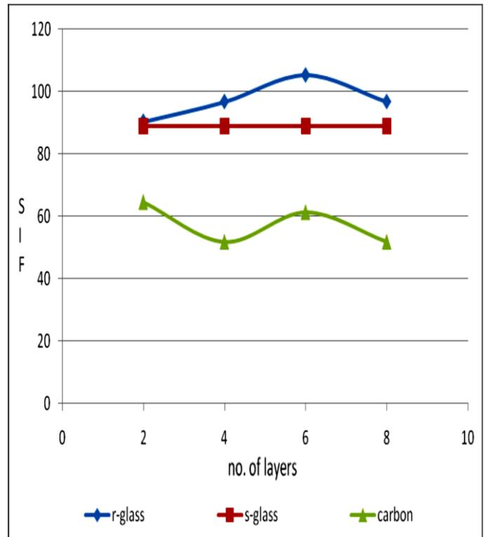
Fig. 27. Variation of Stress Intensity Factor (SIF) with increasing number of layers
