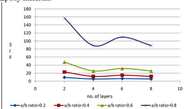
Fig. 22. Variation of Stress Intensity Factor (SIF) with increasing number of layers
