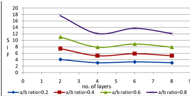
Fig. 21. Variation of Stress Intensity Factor (SIF) with increasing number of layers
