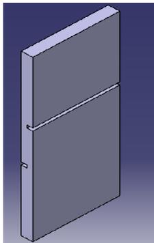
Fig. 17. Model of the plate with a double notch
