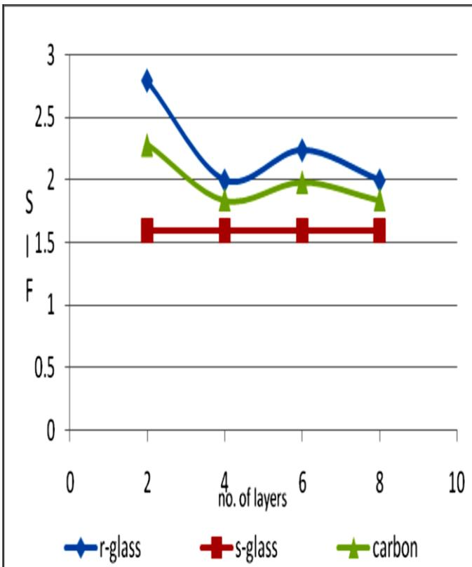
Fig. 29. Variation of Stress Intensity Factor (SIF) with increasing number of layers
