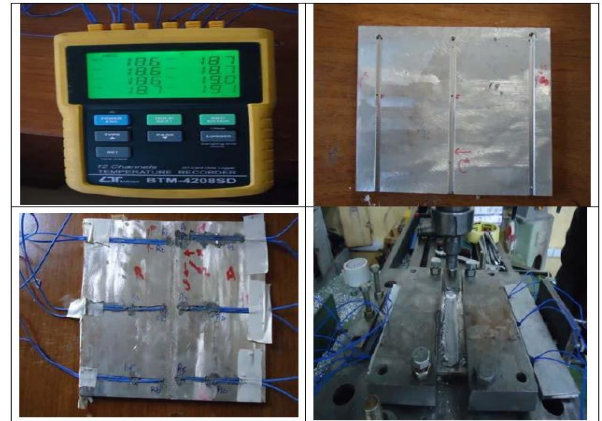
Figure-4. Temperature recorder and hole drill thermocouple position on workpiece.
