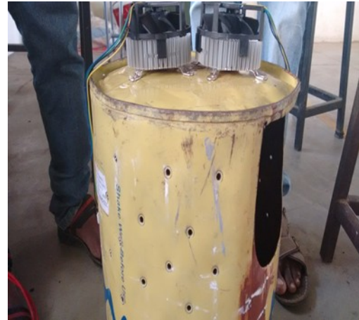
Figure 12 Drilled cylindrical drum stove
