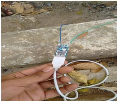
Figure.13 DC-DC step up converter
