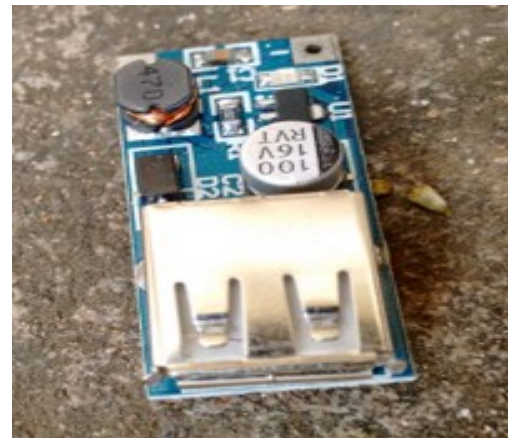
Figure.3 DC-DC Step up converter
