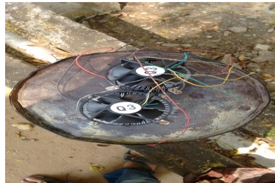
Fig.13 TEG module setup after the cooking or burning
