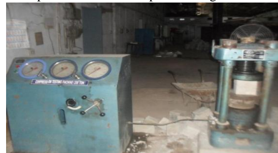
Test Set-up for measuring Compressive Strength of SFRSCC Cube Specimen:- The average of three specimens for compressive strength is given in Table 4.3 and the corresponding graph is given in Figure.
