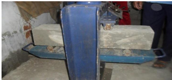
Test Setup for measuring Flexural strength of beam Specimen
