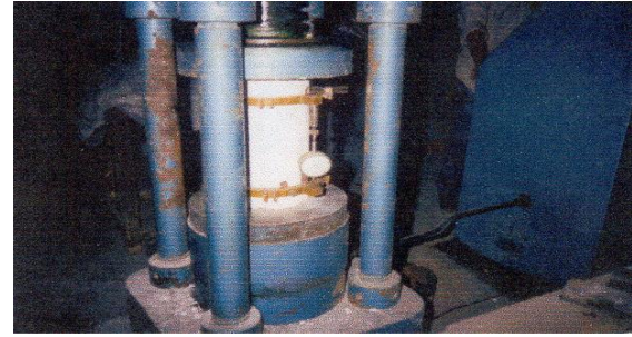
Modulus of elasticity tested with cylinder Specimen attached to extensometer
