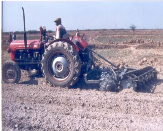
Fig 3. Soil flyash mixing with a disc harrow
