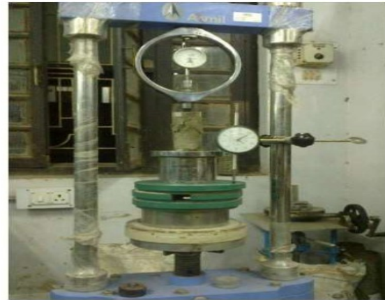
Fig.1 Photographic image showing the test setup of UCS
