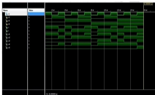
Figure.10: Simulation result of modified 4-2 compressor
