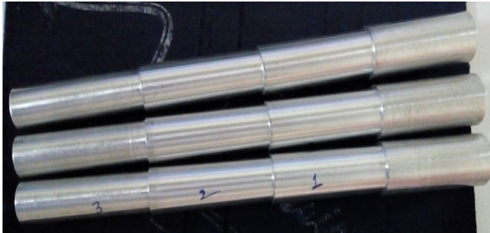
Fig - Prepared Work pieces after cylindrical Grinding Process
