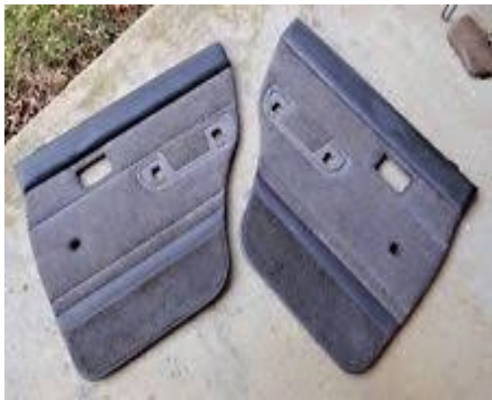
Figure1. The internal door panel of Toyota Corolla DX model vehicle
