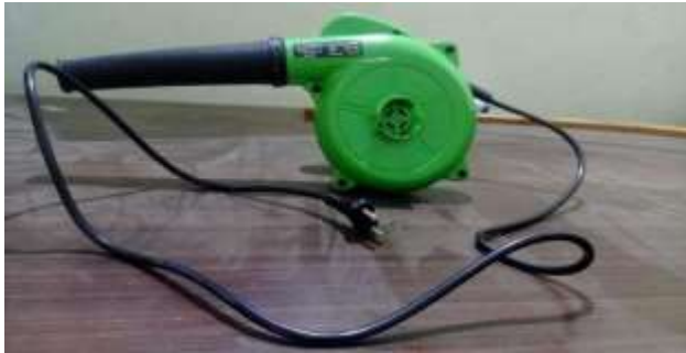
Figure 9. Air Blower of 500W to supply air in setup.
