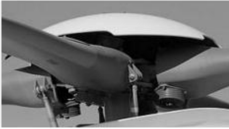
Fig. 2: Rigid rotor system
