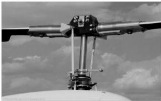
Fig 3: Semi-rigid rotor system
