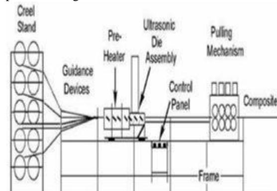
Precisely machined and often chromed, the die is heated to a constant temperature, and may have several zones of temperature through-out its length, which will cure the thermosetting resin. The profile that exits the die is now a cured Pultruded Fiber Reinforced Plastic (FRP) composite. This FRP pro -file is pinched and pulled by a “gripper” system. At the end of the pultrusion machine there is a cut-off saw. Pultruded profiles are cut to the specific length and stacked for
