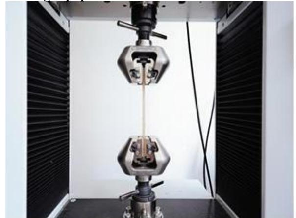
Figure.3: Laminate is fixed between jaws for tensile loading.
