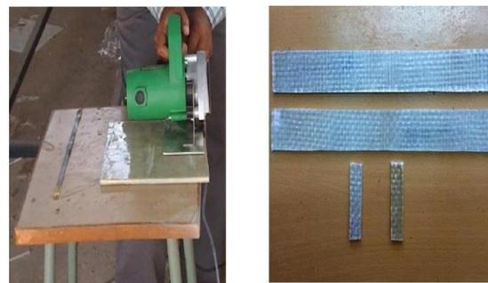
Figure.1: Cutting the laminate into a required dimension.
