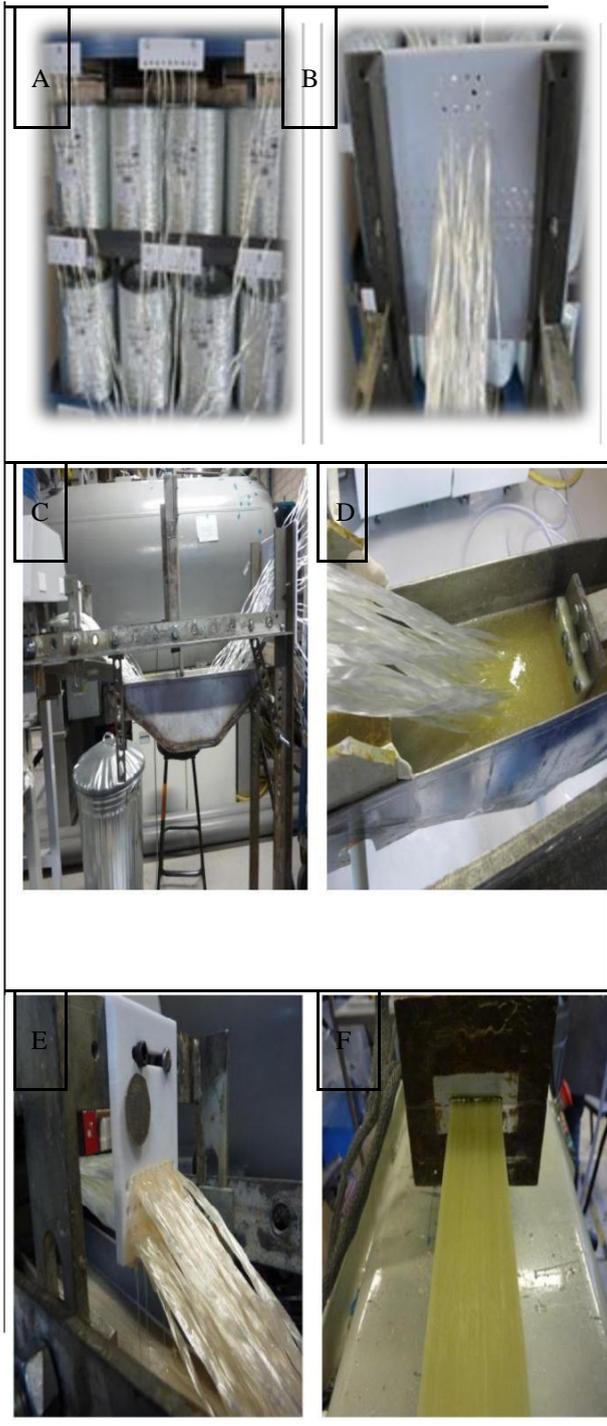
The resin bath was secured to the frame of the pultrusion machine. After securing the resin bath in position, the fibre rovings were threaded through the plunger, forming plates and the die. In order to pass the dry rovings through the die, one roving was threaded with the help of a brass wire. The remaining
