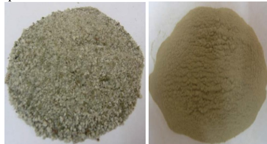
Figure 1. The granulated blast furnace (GBF) slag powder used for synthesis of Aluminium-granulated blast furnace slag (GBF) slag composites (a) As received condition; (b) After crushing and grinding condition.
