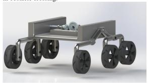
The locomotive duties were handled by six motors incorporated in the legs of the vehicle. the motors are 12V, with 6 mm shaft diameter, brushless DC motor capable of churning out 30 rpm maximum output. Analysis over multiple terrains, like marshy land, rocks, sand, depicted this motor and wheel combination to be suitable concerning the sustainability of the chassis and the frame, consisting of the arm, the Arduino microcontroller and all its peripherals acting as payload.
