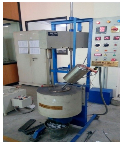
Fig. 4: stir casting Furnace
