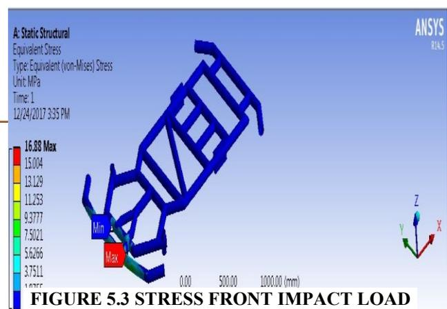
FIGURE 5.3 STRESS FRONT IMPACT LOAD
