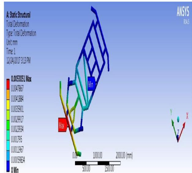
Figure 5.2 Total deformation in general load conditions
