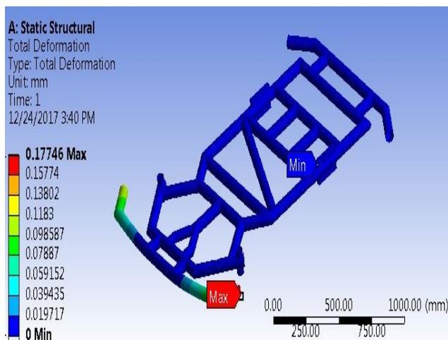
**FIGURE 6.4 TOTAL DEFORMATION IN FRONT IMPACT**
