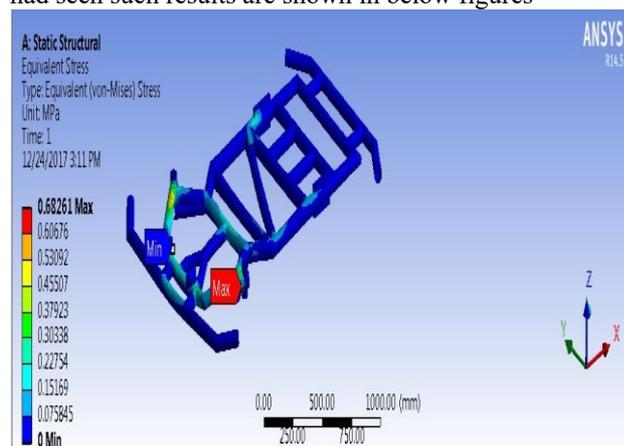
FIGURE 5.1 STRESS IN GENERAL LOAD CONDITIONS
