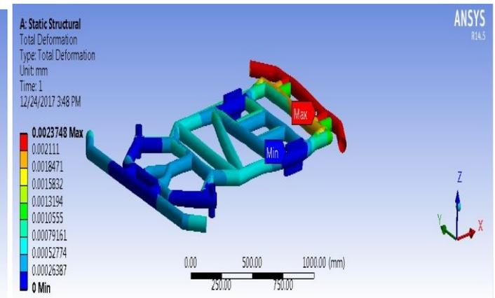
**Figure 6.6 Total deformation in side impact**
