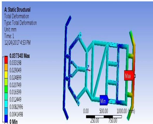
Figure 6.8 Total deformation in rear impact
