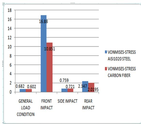
Figure 7.1 Stresses in static analysis graph
