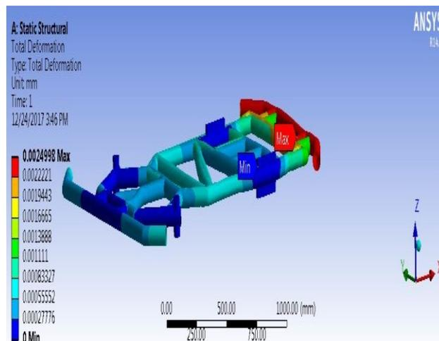
Figure 5.5 deformation in a rear impact
