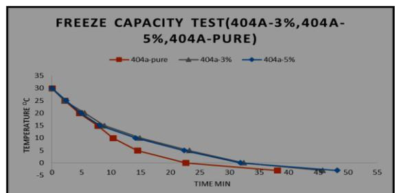
Fig.10. Freeze Capacity Test for R404a-pure, 3% & 5% oil
