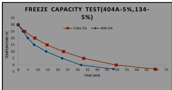
Fig.8. Freeze Capacity Test for R404a-5% oil & R134a-5% oil
