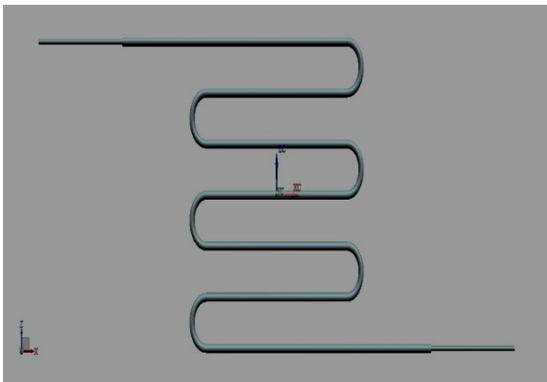
Fig.2. Double tube condenser design (nx8.0)
