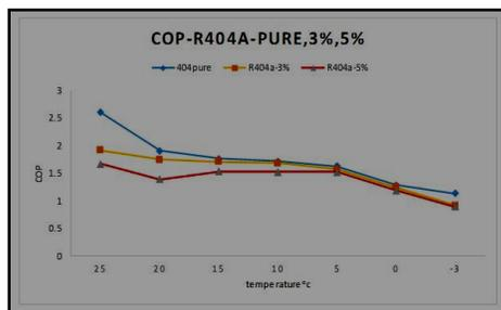
Fig.12. COP Test-R404a-pure, 3%&5% oil
