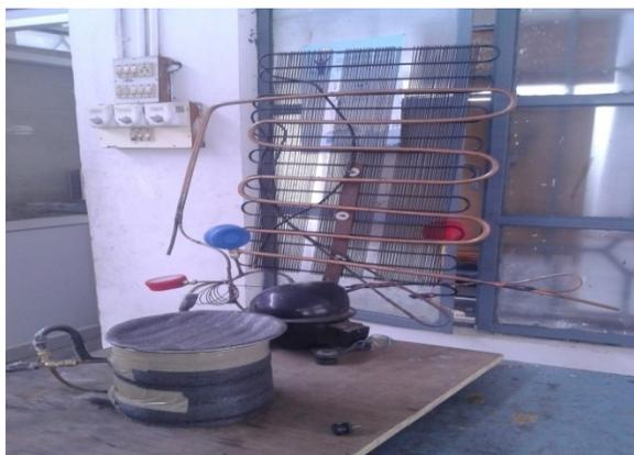
Fig.4 Experimental setup of double tube condenser
