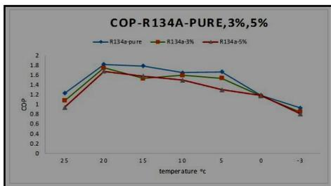
Fig.11. COP Test-R134a-pure, 3%&5% oil
