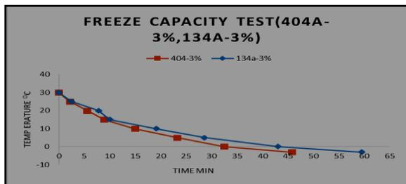
Fig.7 Freeze Capacity Test for R404a-3% oil & R134a-3% oil
