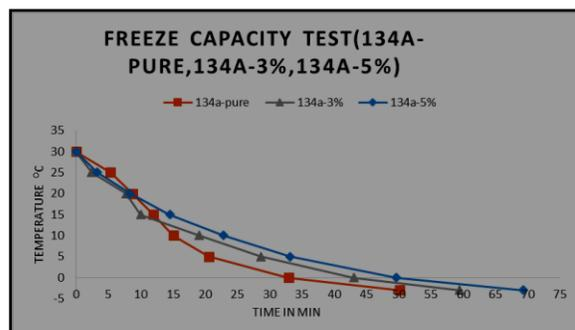
Fig.9 Freeze Capacity Test for R134a-pure, 3%oil & 5% oil
