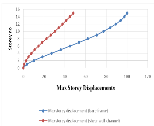
Figure 13. storey displacement for a 15 storied bare frame and with channel shear wall
