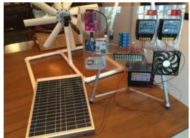
**Fig.12 Hardware implementation of LV grid**
