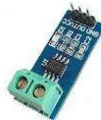
The ACS712 is provided in a small, surface mount SOIC8 package. The leadframe is plated with 100% matte tin, which is compatible with standard lead (Pb) free printed circuit board assembly processes. Internally, the device is Pb-free, except for flip-chip high-temperature Pb-based solder balls, currently exempt from RoHS. The device is fully calibrated prior to shipment from the factory.
