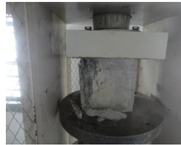
Figure 4: Cubes testing for Compressive strength (1% fibre)
