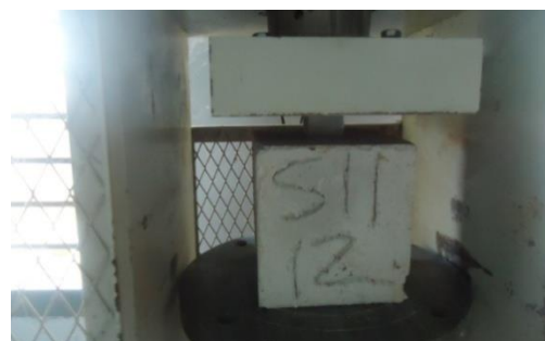
Figure 5: Cubes testing for Compressive strength (2% fibre)
