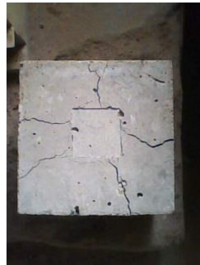
Plate 10: Failure mode of cube using 47.4mm square plate
