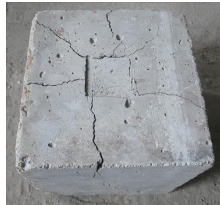
Plate 9: Failure mode of cube using 38.7mm square plate
