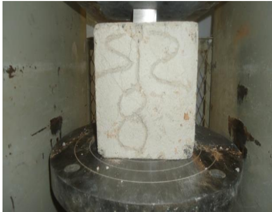
Plate 7: Cubes testing for bearing strength using 47.4mm square plate
