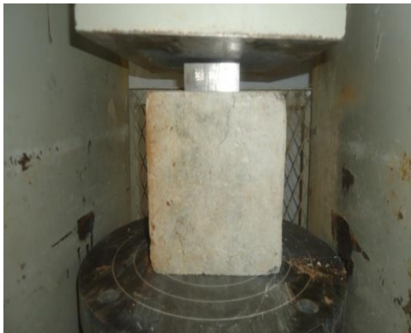
Plate 10: Failure mode of cube using 47.4mm square plate
