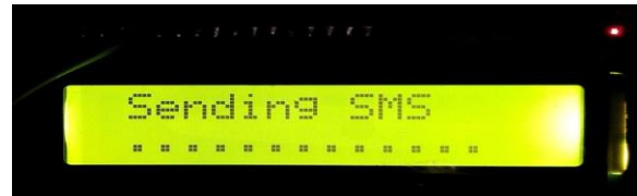
Figure 7. Indication of status of GSM module while sending SMS
