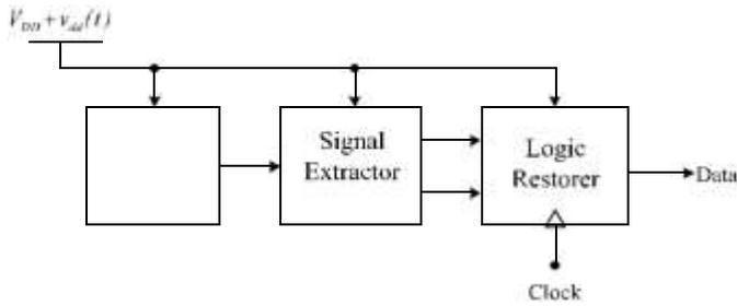
Fig. 2. Block diagram of the proposed PLC receiver.
