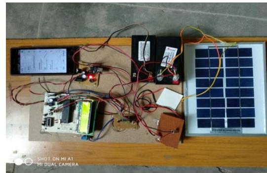
Fig. 8 Proto type of implemented solar e-uniform
