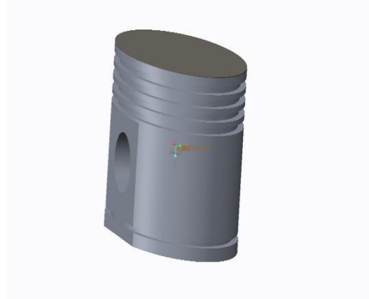
Fig 3.3 Ceramic coated piston with 0.4mm coating layer
