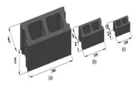
Figure 6: Multiscale stretcher block dimensions: (a) full scale; (b) half-scale; (c) third scale [20]
