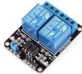
Fig 4.4 2 port Relay board The outputs from the Digital power IC is given to 2 port relay Board which is externally supplied with power. The relay board acts according to the commands supplied by the Digital IC.
