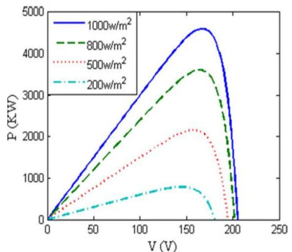
Fig. 2. PV characteristics. input [26].
