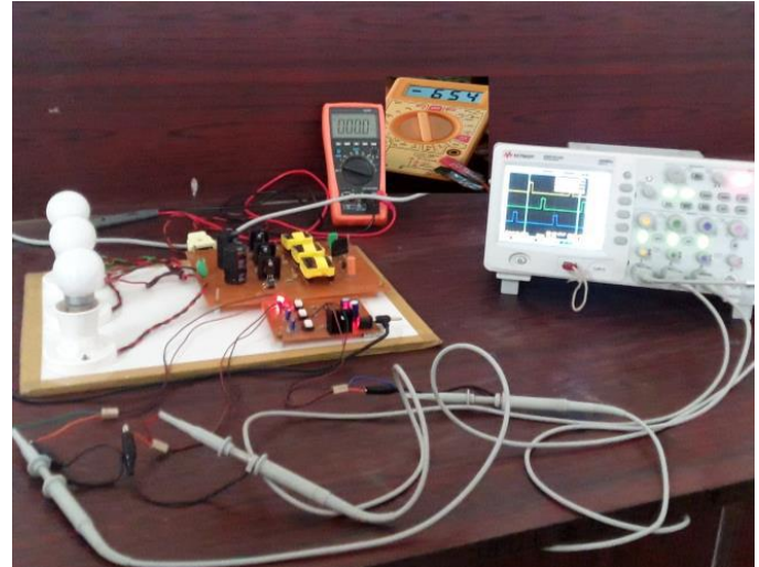
Fig. 14. Experimental setup of a slide mode control dc-dc interleaved boost converter
