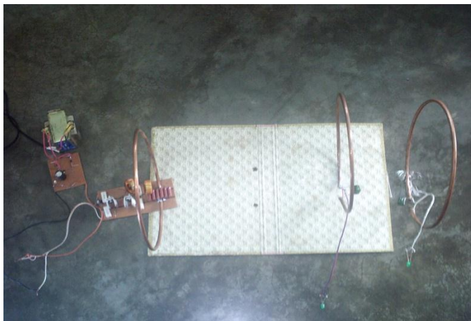
Figure.5 Implementation of wireless power transfer system
