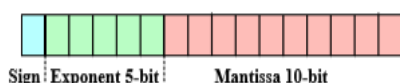
Fig. 1. The OpenEXR format represents pixel values using the "half" data type with 1-bit in the sign field, 5-bit in the exponent field, and 10-bit in the mantissa field in the red, green and blue channels.
