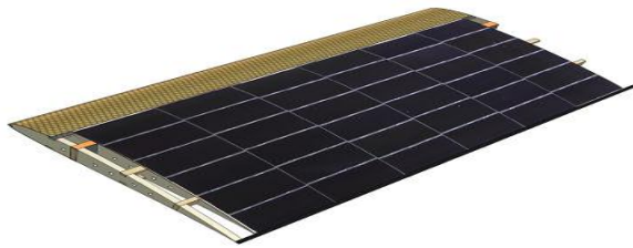
Fig 2: View of the integration of the solar modules on the wing
