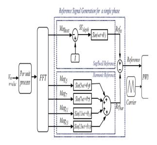
Proposed FFT based reference signal generation method to compensate simultaneous voltage sag/swell and selective voltage harmonics.
