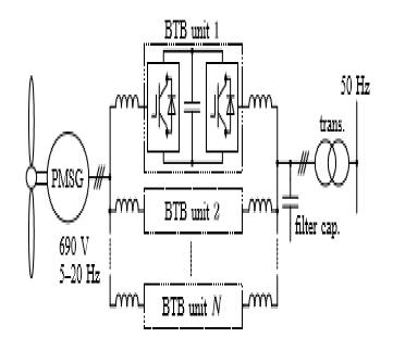
System configuration of a multi-MW WTGS based on a 690-V multi-pole PMSG and multiple BTB converters connected in parallel.
