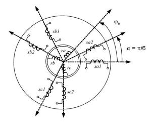
Fig 3.1 : Dual-stator windings induction machine.
