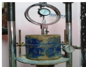
Fig 3.3 California Bearing Ratio Test.
