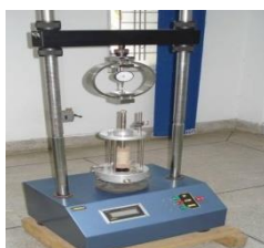
Fig 3.4 Unconfined compression test set up
