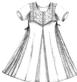
M.S. 9: Kameez has gathers at yoke and sleeves created by pulling draw strings
