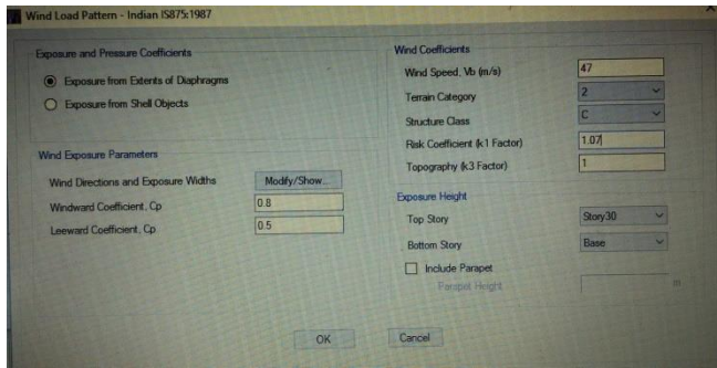
Fig 4.7. Wind load applied for zone 2(Jaipur)
