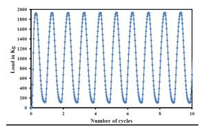
Loading pattern with respect to no of cycles
