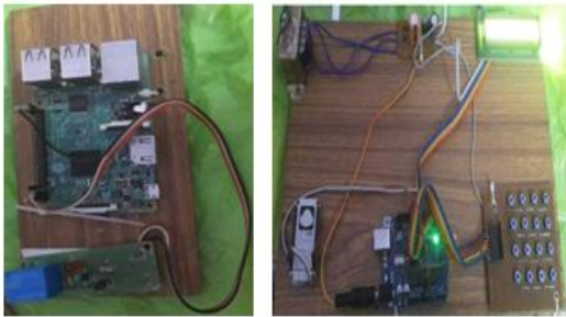
FIG 4. HARDWARE IMPLEMENTATION OF SERVER AND CLIENT
