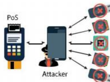
(b) The identity element in FRoDO allows attackers or malicious users to be blacklisted, rendering their coin element unavailable for future transactions.
