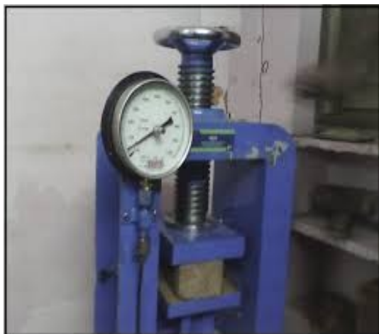
FIGURE 6: TESTING OF SAMPLE BRICKS
