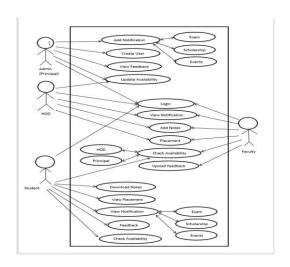
The above shown figure is the use case diagram of SDIT app. This how exactly the working of the application shows. Wherein the principal becomes admin here and has the right to access everything. The HOD and faculty has the permission for accessing only some of the process. And the students can just only view and update feedbacks.
